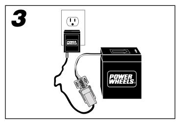
• Plug the charger into a standard wall outlet.
